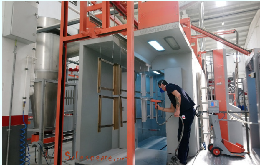
Manual coating for workpieces with difficult corners
